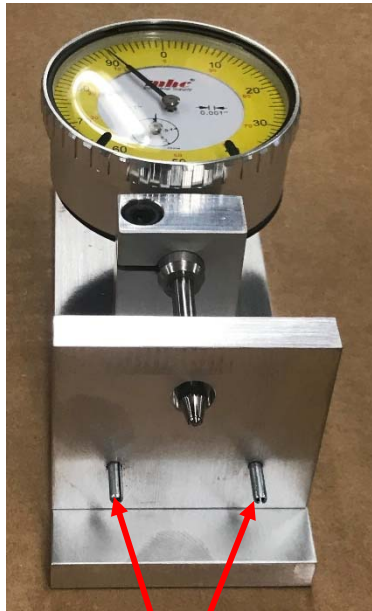
Pins the screw holes in comb blade fit on
