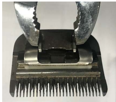
Adjusting socket ears to stop blade rattle
