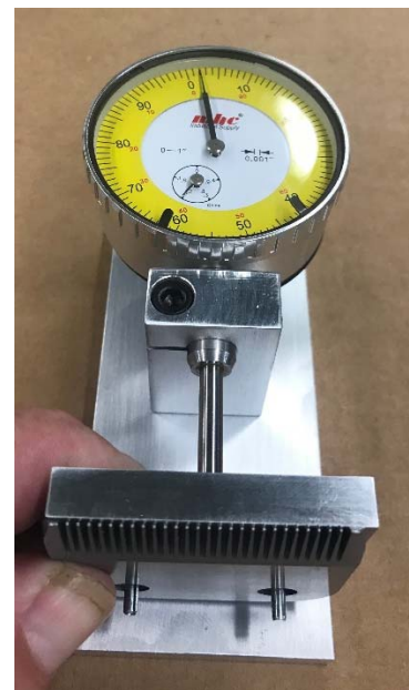
After sharpening needle should be 2 lines from zero
